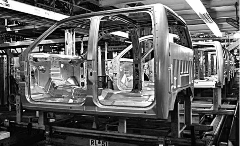
Machines weld truck bodies at a Michigan GM plant.
