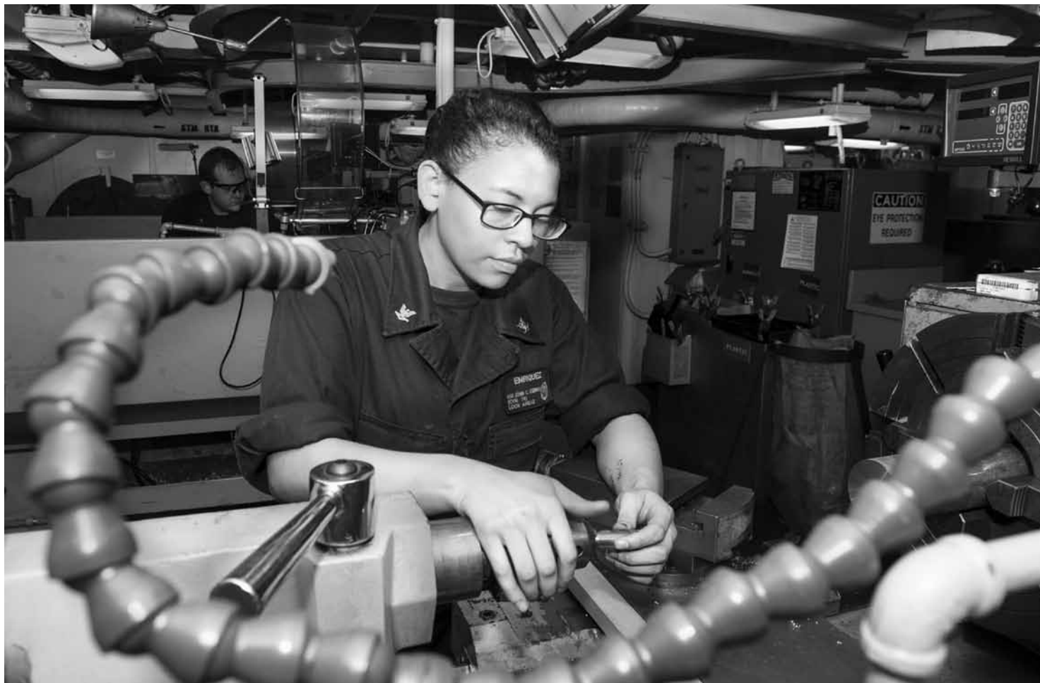
Machinery Repairman 3rd Class Hamali Enriquez from Los Angeles, re-threads a valve stem in USS John C. Stennis' (CVN 74) repair shop. Providing a ready force supporting security and stability in the Indo-Asia-Pacific, John C. Stennis is operating as part of the Great Green Fleet on a regularly scheduled 7th Fleet deployment. U.S. Navy photo by Mass Communication Specialist 2nd Class DeAndrae McDaniel
