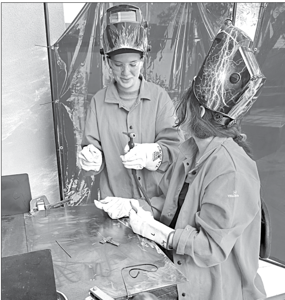
Tatiana Nunez (left) and Francesca Ferrante TIG (Tungsten Inert Gas) welding the Hollywood Sign for the art car. Photo by Jason Kartez.
