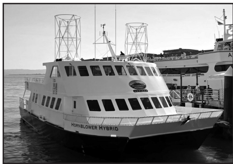
Pictured: The recently retrofitted Hornblower ferry to Alcatraz and Angel islands in San Francisco, which runs on several alternative energy sources, including a hybrid diesel-electric system powered by solar cells and wind turbines right on deck. Image by John K, courtesy Flickr.
