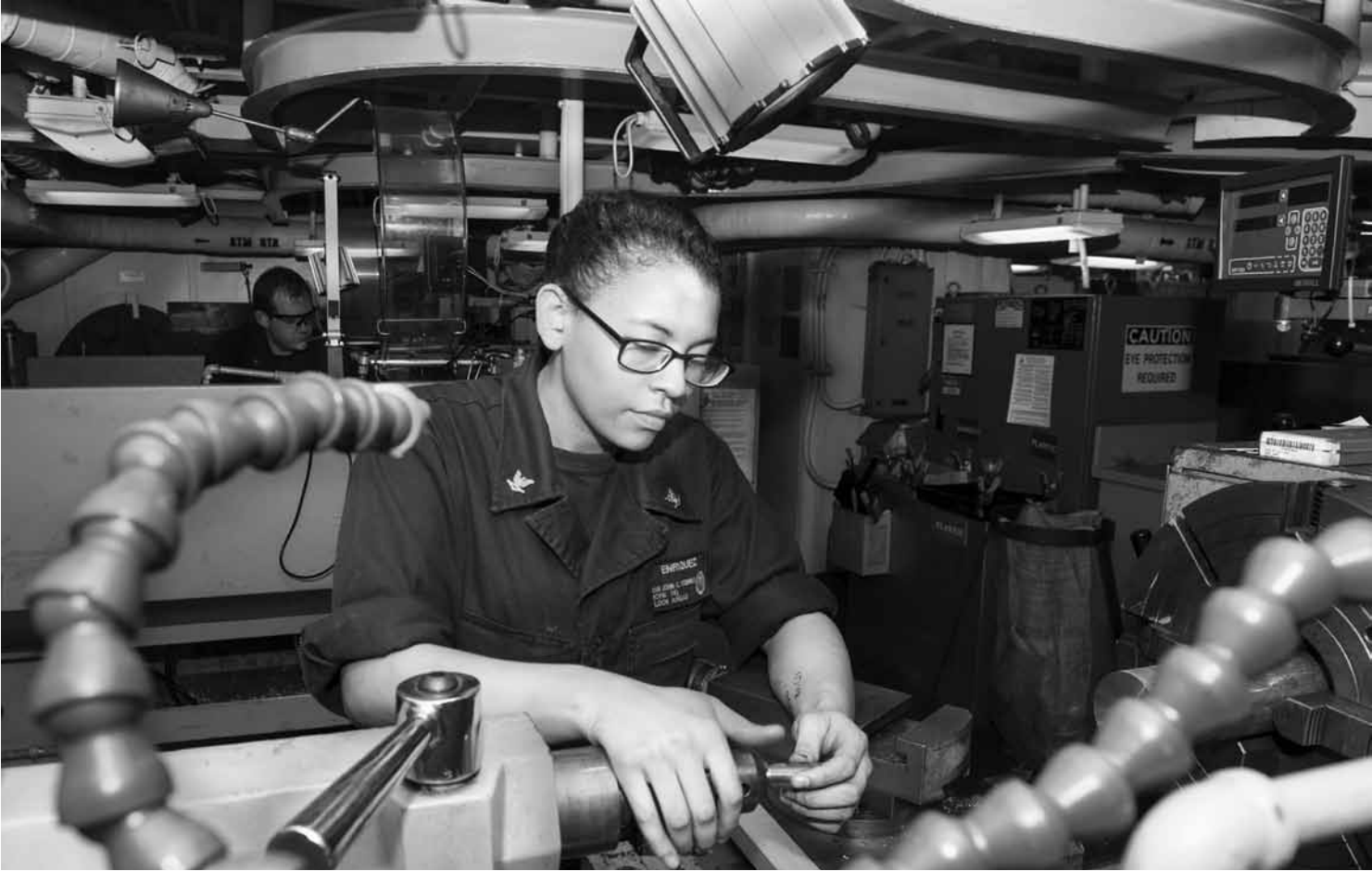
Machinery Repairman 3rd Class Hamali Enriquez from Los Angeles, re-threads a valve stem in USS John C. Stennis’ (CVN 74) repair shop. Providing a ready force supporting security and stability in the Indo-Asia-Pacific, John C. Stennis is operating as part of the Great Green Fleet on a regularly scheduled 7th Fleet deployment. U.S. Navy photo by Mass Communication Specialist 2nd Class DeAndrae McDaniel
