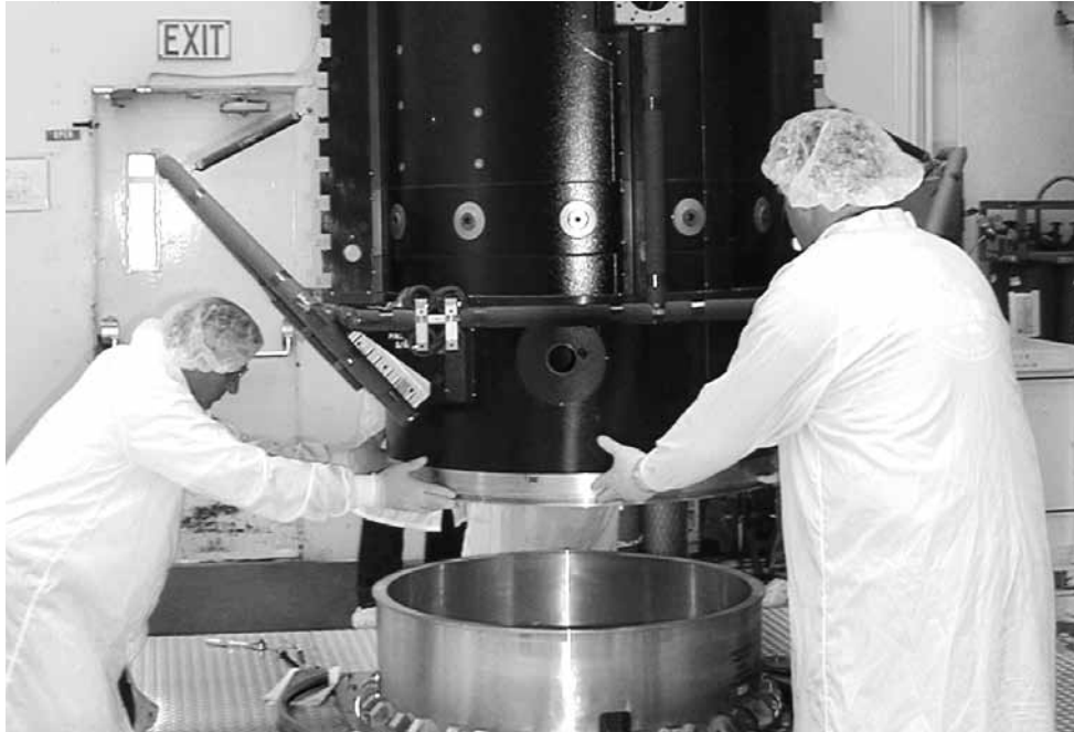
The Dawn Spacecraft being assembled. Dawn was made to orbit the large asteroid Vesta and the dwarf planet Ceres, and was launched in 2007. It has since sent back enough data that scientists can map the surface of Ceres. Photo credit: NASA/JPL.
