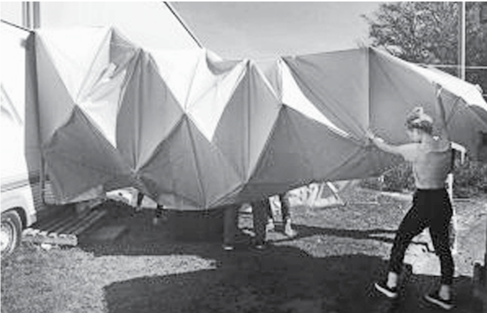
The prototype was deployed and tested to extreme conditions on the 20th of April during the EuroMoonMars2018 simulation at ESA – ESTEC. The origami structure was designed as a gateway and sub-system between the exo-habitat, airlock system and exo-laboratory. Credit: Anna Sitnikova.
